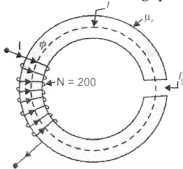
Figure 11 (a) Magnetic circuit I
